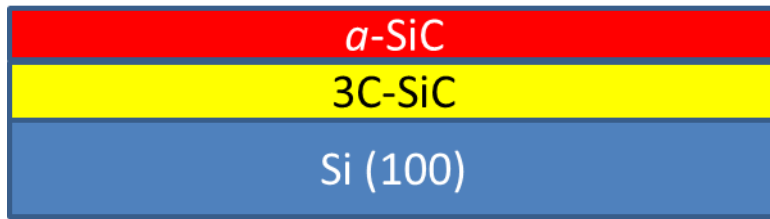
Figure 2.7: Cross-section showing the structure of type III a -SiC developed for testing in this research. The a -SiC was \sim 300 nm thick, deposited on \sim 6.2 \mu\text{m} 3C-SiC and grown on 500 \mu\text{m} thick Si (100) substrate.
